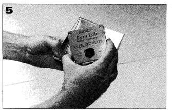
With the transducer and display unit installed, the last main component to install is the accelerometer. As shown here, it can be rotated in its mounting bracket so it can remain exactly parallel to the imaginary line that travels from the front to the rear of the car—regardless of the bracket's mounting position.
