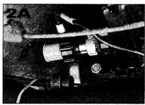
we didn't install the cable. We left the cap on the end of the transducer and tiewrapped the cable out of harm's way (photo 2A). With the dyno, the Chevelle now has an accurate speedometer. If you have a race car with no speedo hookup on the transmission or anywhere else, then DynoLab offers an optional photo speed transducer. It uses an infrared light beam and reflective tape on the surface of the driveshaft to measure vehicle speed.
