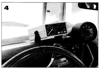
Select a mounting position for the display unit that's within view of the driver. We used double-sided tape to mount it on the Chevelle's dash, just to the right of the driver. The dyno can also be mounted to the steering column with a hose clamp passing through the two holes in the mounting bracket.
