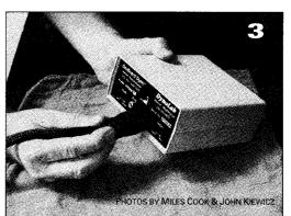
Plug the wiring harness end (with the eight-nin Weather Packtype connector) into the back of the computer/ display unit. A click will indicate the connector is locked in place. The heavy red lead
